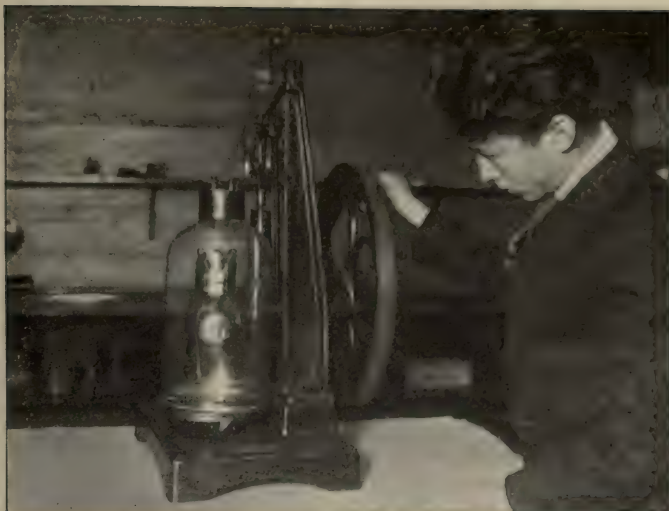
FIG. 97. When the air is pumped out of the jar, you cannot hear the bell ring.
